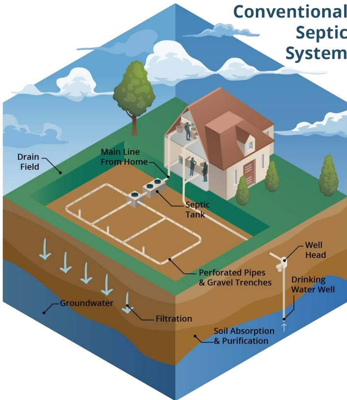
During floods or heavy rains, the soil around the septic tank and in the drainfield become saturated, or water-logged, and the effluent from the septic tank can't properly drain through the soil. Special care needs to be taken with your septic system during and after a flood or heavy rains.
