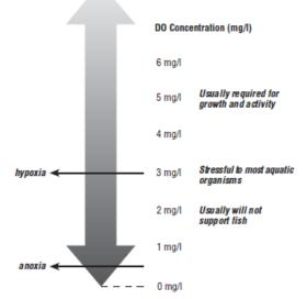
Dissolved oxygen in the water. A minimum DO concentration of 5 mg/l is usually necessary to fully support aquatic life. Image credit: EPA. Volunteer Estnary Monitoring: A Methods Manual
